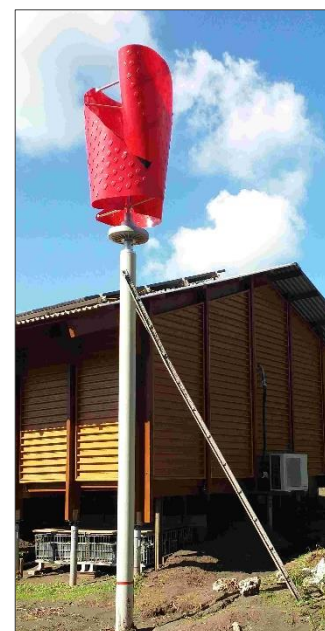
Figure 3.9: Vertical- Axis Wind Energy, Tanna Photo: J Salong, May 2016
